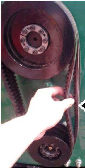
If you can press the belt more than 2cm, then need to tighten the belt.
