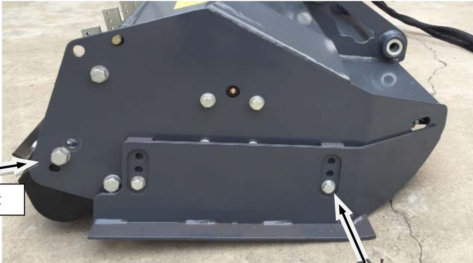
2. If your tractor 3 point hitch is CAT 1, then remove these bushing. If your tractor 3 point hitch is CAT 2, then keep these bushing.
