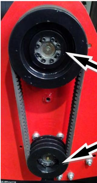
Loosen these bolt to adjust the belt wheel's position on the shaft, always keep the upper and lower belt wheels are vertical in line.
