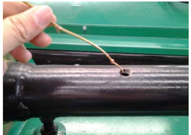
Use a stick to test if oil in the transmission and shaft tube every month.
